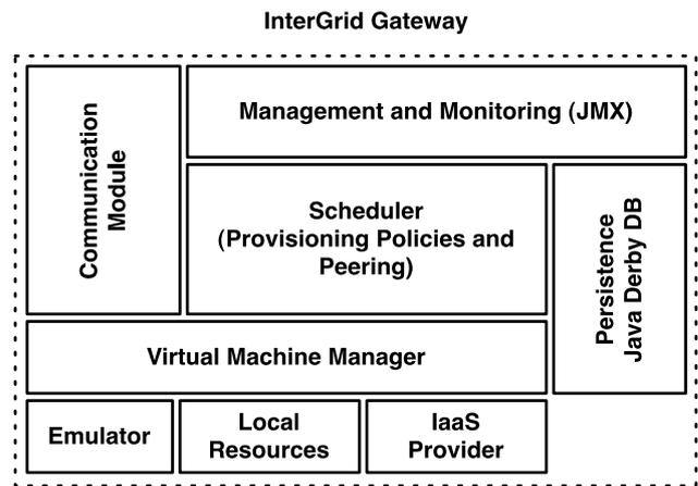
Fig. 2 Main components of the IGG
